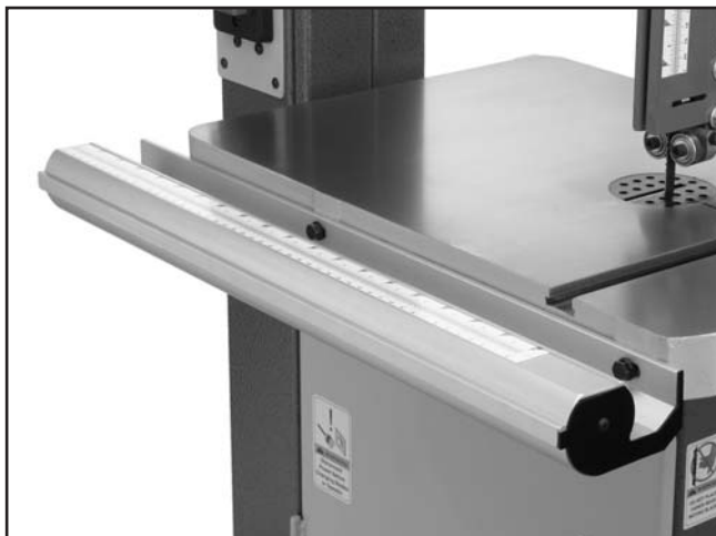
Figure 12. Installed fixed rail.
